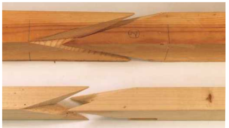
▲ Pic.9 The joints pulled apart. This is a joint that can be used for making long boat hook poles, so I am told!
